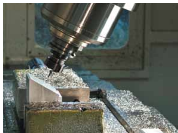
Work in inclined planes
