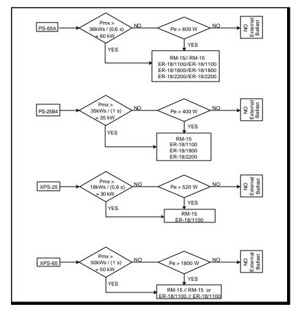
Check that the external resistor meets the Wmx and Pe requirements of the application.
